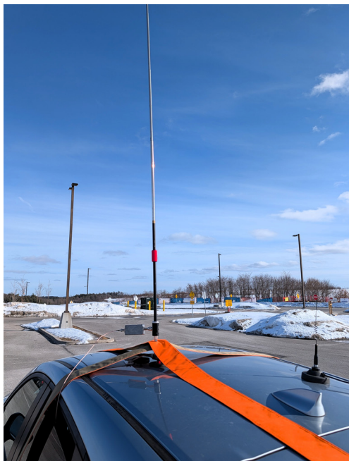
Figure 10 — The Chameleon CHA FSR with the Chelegance MC-750 antenna installed on the mobile roof using a magnetic mount.
